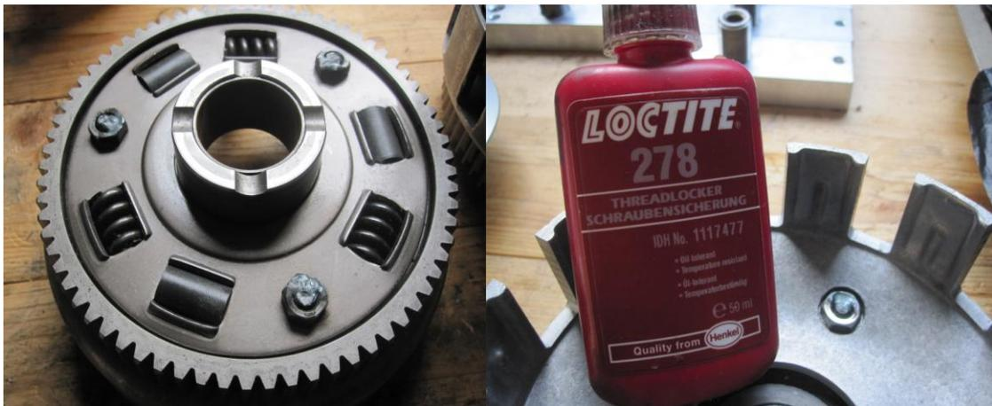
**DO NOT INSTALL THIS KIT WITHOUT USING LOCTITE 278 ON THE THREADS!!!!**
